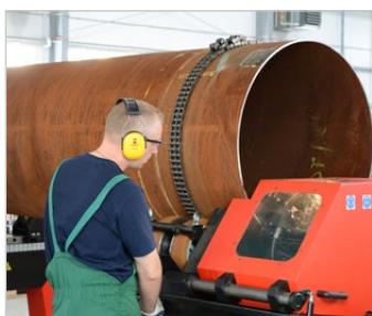
Shields and internal lighting increase safety and comfort of the operator
