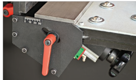
Simple setting of bevel width
