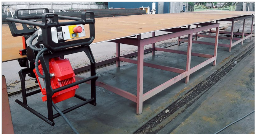
ABM-14 runs along a plate automatically
