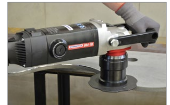
Rounding off curved edges
